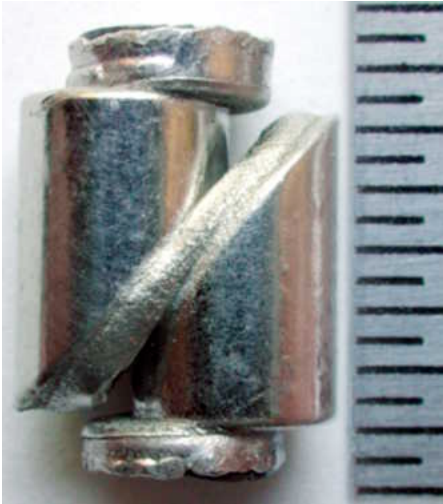
Sample (& Pt jacket) after deformation
